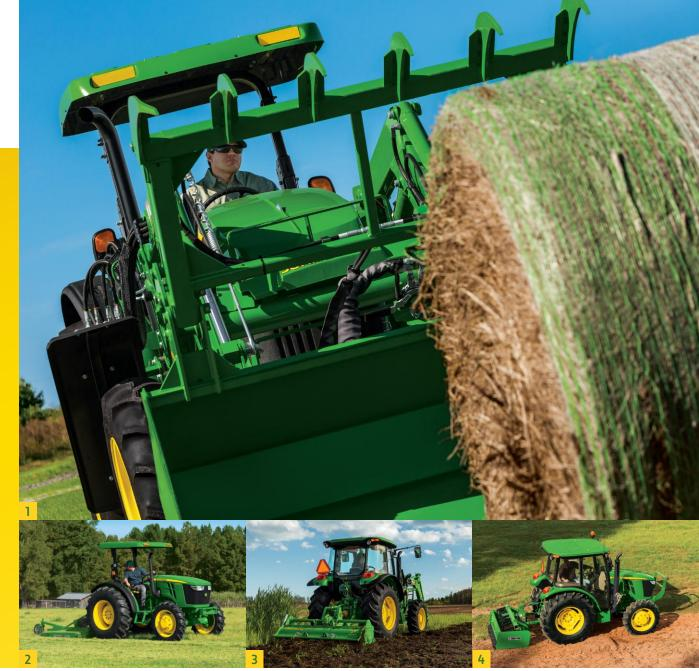
5085E Tractor shown with H240 Loader and 3rd Function Grapple Bucket. 2. 5075E Tractor shown with Canopy and Frontier RC2072 Rotary Cutter.
