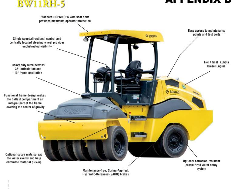
The BW11RH-5 pneumatic tired roller is one of the most versatile machines in the Bomag line. This roller achieves its high compaction performance through the combined effect of vertical pressure with the horizontal forces directed to all sides under each of the nine, overlapping tires.
