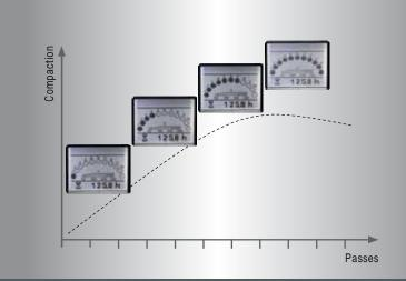
ECONOMIZER knows when full compaction is reached: The lighting strip shows the degree of compaction and warns of over-compaction.
