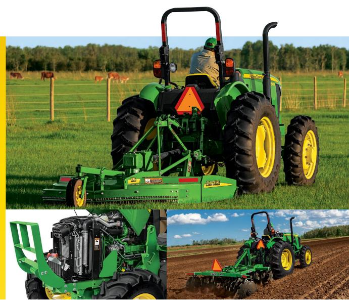
The one-piece tilting hood allows easy access to to service items like the air filter, engine oil checks, and more. Plus, ground-level fluid fills make regular maintenance a snap.
