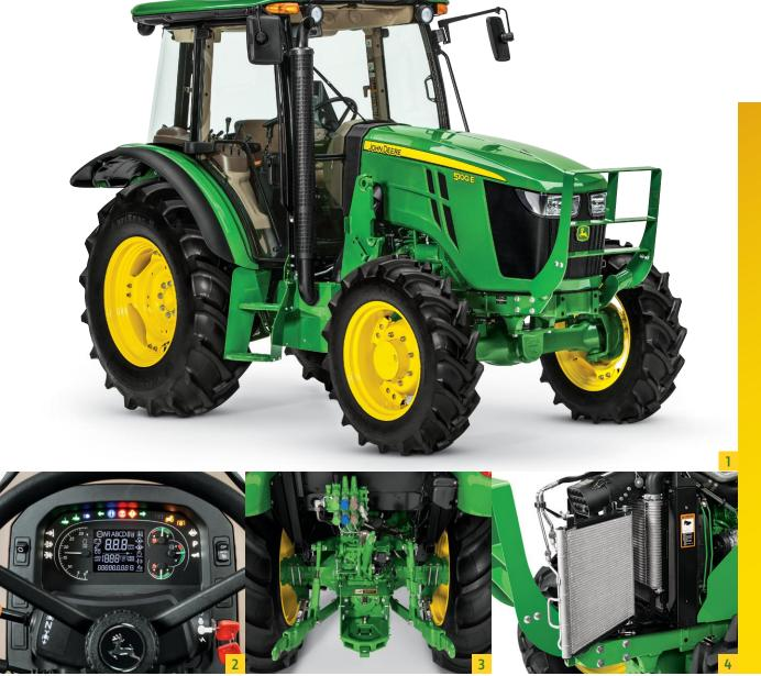
1. New sloping hood on 5E 4 cylinder. 2. New LCD instrument cluster. 3. New standard sway bars and telescoping draft links. 4. New slide out condenser, radiator screen, tilt-able charge air cooler, and slide out condenser on 4 cylinder cab models.
