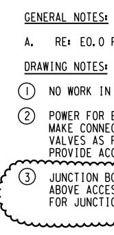
A. RE: EO.O FOR MORE GENERAL NOTES, SYMBOLS, AND ABBREVIATIONS. ○ NO WORK IN THIS ROOM/AREA. 2 POWER FOR ELECTRONIC FLUSH VALVE CONTROL POWER TRANSFORMER. MAKE CONNECTION TO TRANSFORMER ABOVE CEILING AND TO FLUSH VALVES AS REQUIRED IN MANUFACTURERS INSTALLATION INSTRUCTIONS. PROVIDE ACCESS PANEL IN DRYWALL CEILING. JUNCTION BOX AT 18" A.F.F. WITH EMPTY I 1/4" CONDUIT AND PULL CORD TO ABOVE ACCESSIBLE CEILING FOR FUTURE USE. PROVIDE BLANK COVER PLATE FOR JUNCTION BOX. ..... ·····
